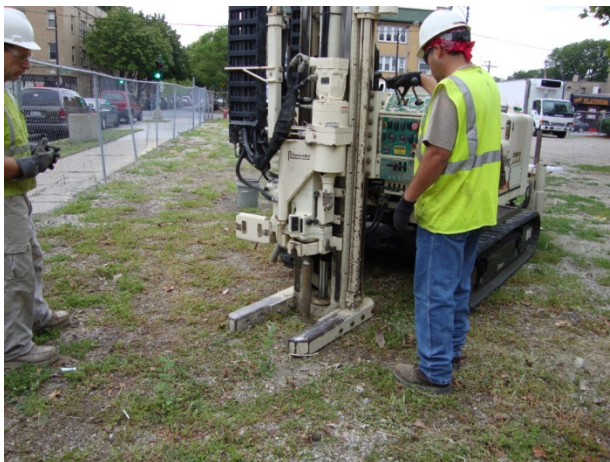
Soil Sampling with a Geoprobe
